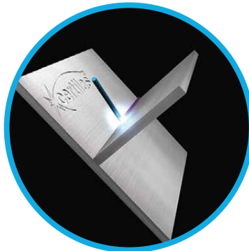
Axis of Weld Horizontal Flat Position ASME : 1F ISO: PA
